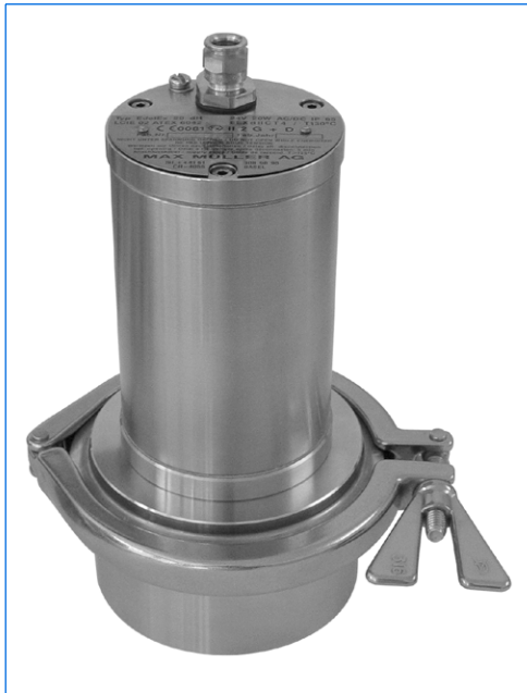
Sightglass light fitting, type EdelEx STERI-LINE 20 dH, 24 V, 20 W, Ex d IIC T4 Gb, Ex t IIIC T130°C Db IP67, Ex II 2 G + D, on metal fused sightglass, DN 100
