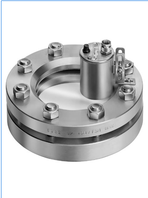
Sightglass light fitting type BKVLR LED DSch1, 24 V, with built-in momentary push-button "D", mounted with tilting hinge "Sch" on sightglass to DIN 28120, DN 100, PN 10, for application "view and light through one assembly".
