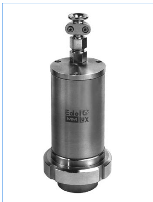
Sightglass light fitting type EdelEx 10 dH R50 K1, 10 W, 230 V, Ex d IIC T4 Gb, Ex t IIIC T130°C Db IP67, Ex II 2 G + D, with intermediate flange collar fixation "R", mounted onto a screwed sightglass similar to DIN 11851, PN 6, DN 50.
