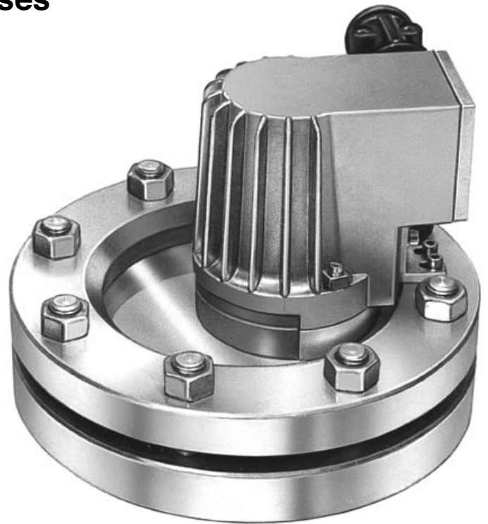
Type KEL 20 deH W, Ex d e IIC T4 Gb, Ex t IIIC T130°C Db IP67, Ex II 2 G + D, 230 V, 20 W, mounted on circular sightglass to DIN 28120, DN 125, PN 10, in 1 port version.
