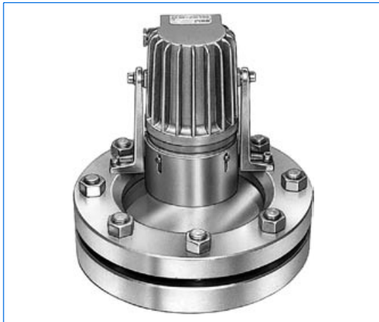
Safe area type KL 100 H Sch B, 24 V, 100 W, with anti-dazzle shield "B", on circular sightglass to DIN 28120, DN 150, PN 10, in version "view and light through one sightglass".
