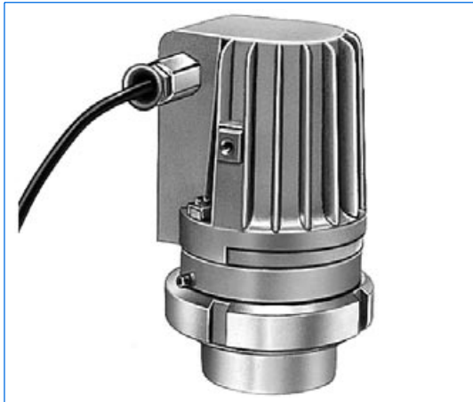
Hazardous area type FKEL 20 dH R, Ex d IIC T4 Gb, Ex t IIC T130°C Db IP67, Ex II 2 G + D, 230 V, 20 W, on screwed sightglass similar to DIN 11851, DN 65, PN 6. Fixation with intermediate flange collar "R".
