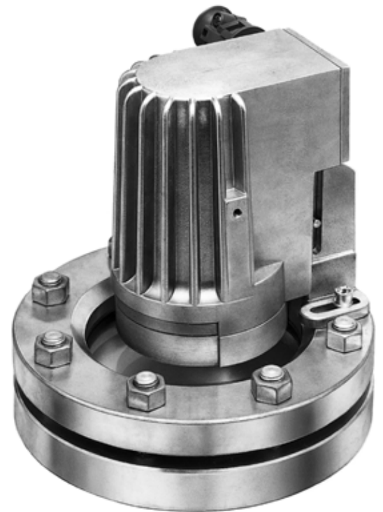
Type PEL 50 deHSch, Ex de IIC T4, Ex tD A21 IP65 T130°C, Ex II 2 G + D, 230 V, 50 W, mounted on circular sightglass to DIN 28120, DN 125, PN 10, in 2 port version.
