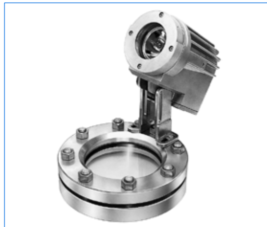
Type PEL 20 deH Sch, 230 V, 20 W, Ex de IIC T6, Ex tD A21 IP65 T80°C, Ex II 2 G + D, mounted on circular sightglass to DIN 28120, DN 125, PN 10, in 1 port version
