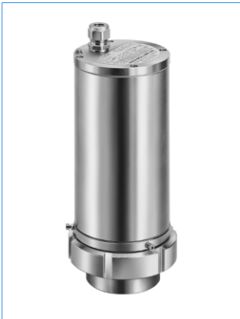
Sightglass light fitting type EdelEx G20 dH R 80 K1, 20 W, 230 V, Ex d IIC T5, Ex tD A21 IP65 T95°C, Ex II 2 G + D, with intermediate flange collar fixation "R 80" mounted on a screwed sightglass similar to DIN 11851, PN 6, DN 80.
