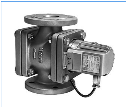
Hazardous area type FKEL 5 dH WM, Ex de IIC T6, Ex tD A21 IP65 T80°C, Ex II 2 G + D, 230 V, 5 W, with opal glass "M", on pipeline flow indicator DN 50.
