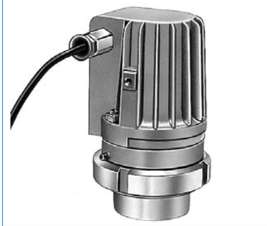
Hazardous area type FKEL 20 dH R, Ex d IIC T4, Ex tD A21 IP65 T130°C, Ex II 2 G + D, 230 V, 20 W, on screwed sightglass similar to DIN 11851, DN 65, PN 6. Fixation with intermediate flange collar "R".
