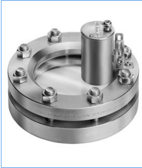
Sightglass light fitting type KLR 50 HSch, 50 W, 24 V, mounted with tilting hinge "Sch" on sightglass to DIN 28120, DN 100, PN 10, for application "view and light through one assembly".
