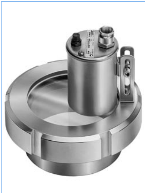
Sightglass light fitting type BKVLR 50 HDSch1, 50 W, 24 V, with built-in momentary push-button "D" mounted with tilting hinge "Sch1" on screwed sightglass similar to DIN 11851, DN 100, PN 6, for application "view and light through one assembly".
