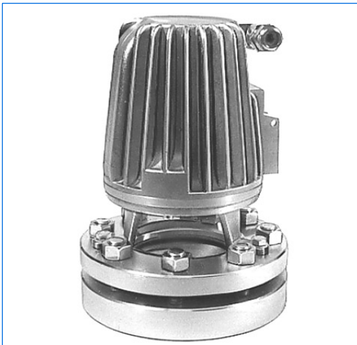
VETROLUX® illuminated sightglass unit, consisting of sightglass to DIN 28120, DN 80, PN 10, with mounted CHEMLUX® light fitting, type F 20dHNsp, 24 V, 20 W, Ex d IIC T5, Ex tD A21 IP65 T95°C, Ex II 2 G + D
