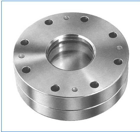
Double glazed safety sightglass similar to DIN 28121, DN 125, PN 10
