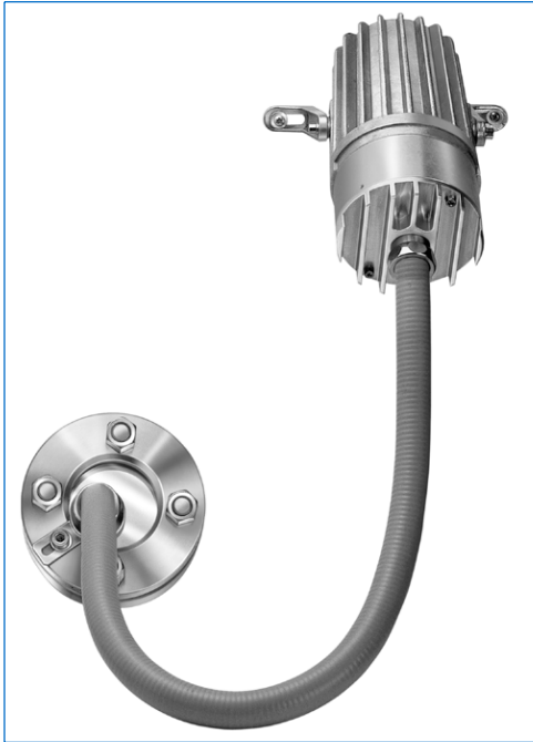
Fibre-optic lightpipe light fitting for use in hazardous areas with built-in timer "V", type fibroLUX® 5035 X1 W2 V, Ex de IIC T4, Ex tD A21 IP65 T130°C, Ex II 2 G + D, 35W, 230V, fixation of the light source by fixation legs "X1", fixation of the lightpipe by universal support "W2" onto sightglass to DIN 28120, DN 40, PN 10
