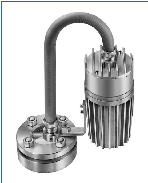
Fibre-optic lightpipe light fitting with built-in timer "U", type fibroLUX® 5035 W W2 U sp, Ex de IIC T4, Ex tD A21 IP65 T130°C, Ex II 2 G + D, 35 W, 12 V DC, fixation of the light source by bracket "W", fixation of the lightpipe by universal support "W2" onto sightglass to DIN 28120, DN 40, PN 10
